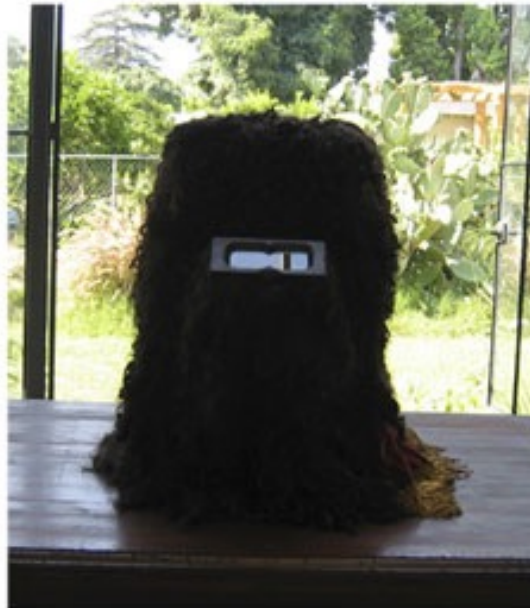
Camera obscura - image projects onto the interior base of the obscura as depicted in Scientific American engraving. Dimensions: Length 26" Height 19 1/2", Width 18"
